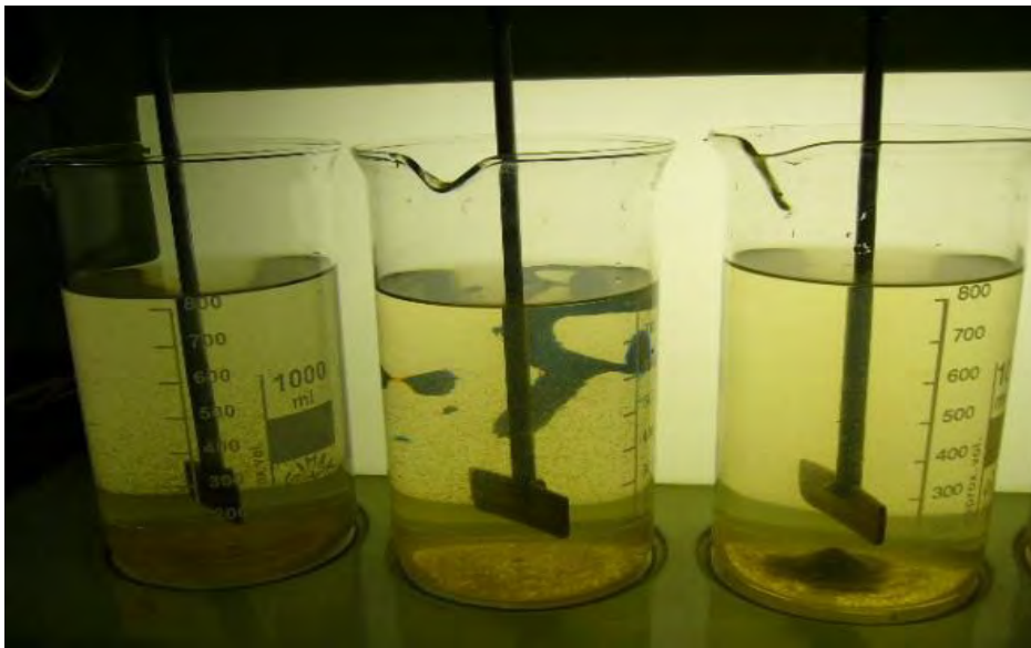
Figure 5: Beaker test showing effect of ballasted floc
