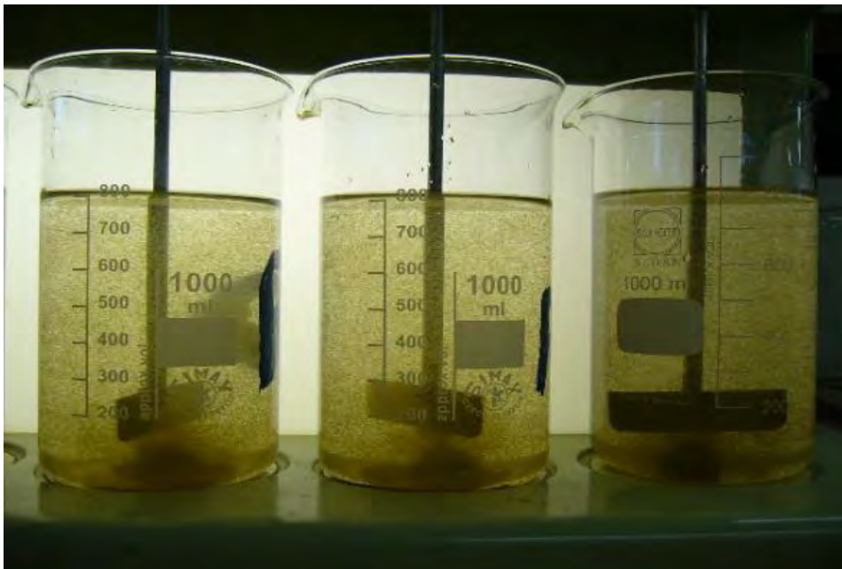
Figure 4: Beaker Test During Flocculation
