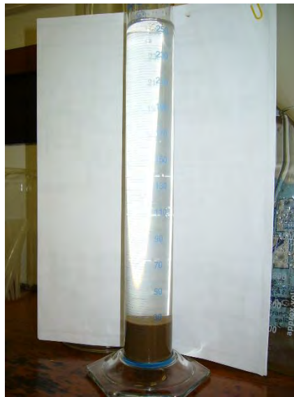
Figure 6: Typical sludge settling test
